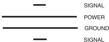
FIGURE 10-30. A common four-layer printed circuit board stackup.
