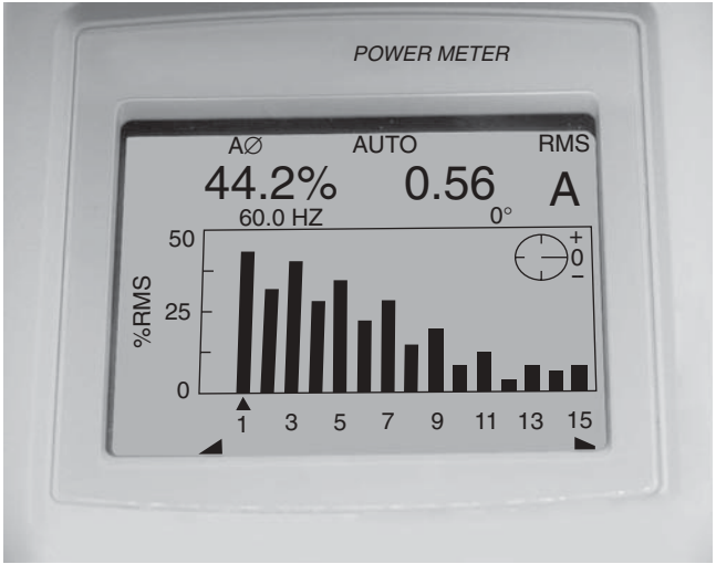
FIGURE 18-31. Harmonic current from of a small switching power supply, displayed on a harmonic meter.
