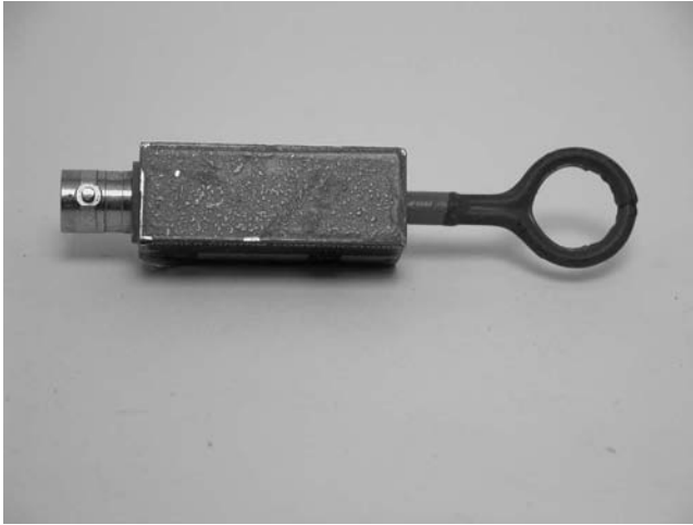
FIGURE 18-5. Small split-shield magnetic field loop probe.
