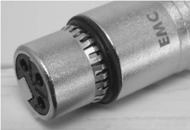
FIGURE 2-42. A female XLR connector (used in pro-audio installations) with spring fingers around its circumference to provide a 360° contact between mating halves of the connector backshell.
