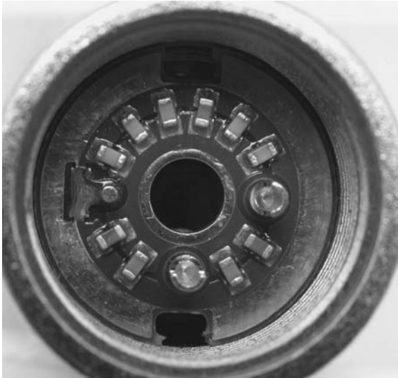
FIGURE 2-48. XLR connector with 10 SMT capacitors between the cable shield and the connector backshell .
