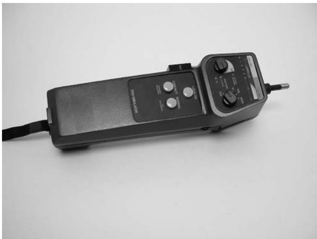
FIGURE 18-28. A small battery powered ESD simulator.
