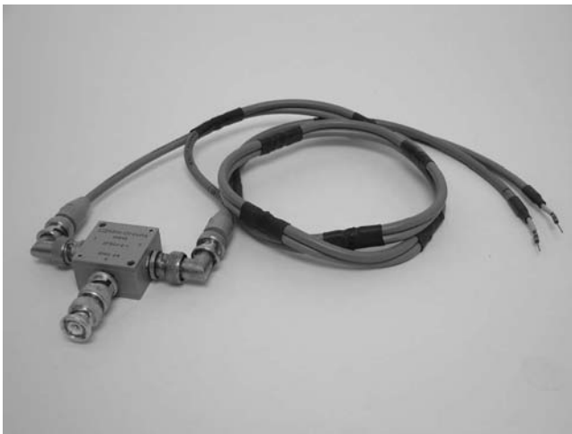
FIGURE 18-9. A home-made X10, passive, differential voltage probe, with a 180^\circ combiner.
